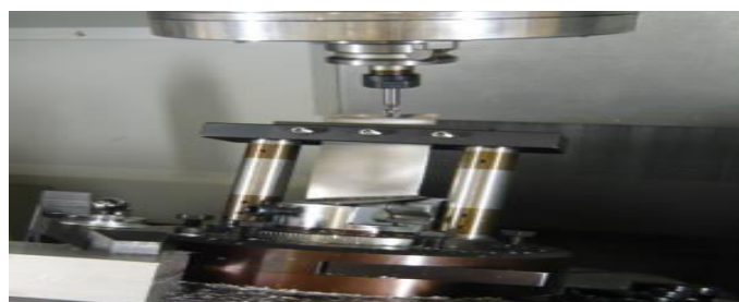
Figure 8: Adaptive CNC blending of repaired air foil tip
